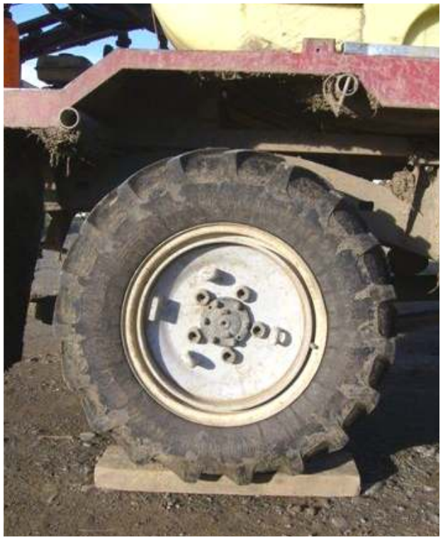
2. Connecting Plate mounted with specific nuts to existing wheel without Clic Dual (road legal)
